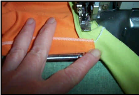
Step 9: when you come to the end of the neckline, fold ribbing to your right, stop stretching, sew straight through all layers.
