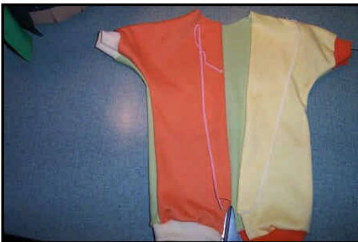
Step 5: serge both front edges for a finished look
