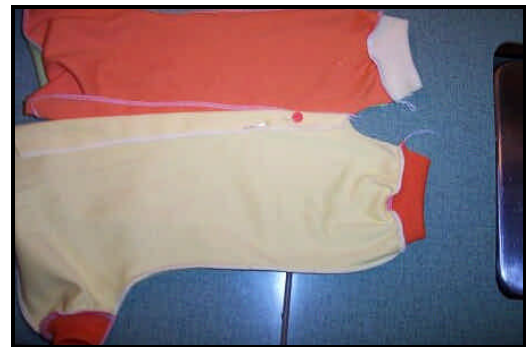
Step 6: inside leg/crotch. With right sides together, adjust/match front and back, fold fronts over, pin.
