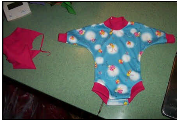
Step 8: weave in all serger tails, turn right side out, ad snaps
